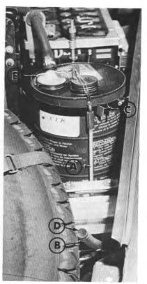
To achieve this start the engine, accelerating slightly to save time. Set the lever **A** (fig. 23 and 24) to position 5 and wait until the car has settled at its maximum height.
